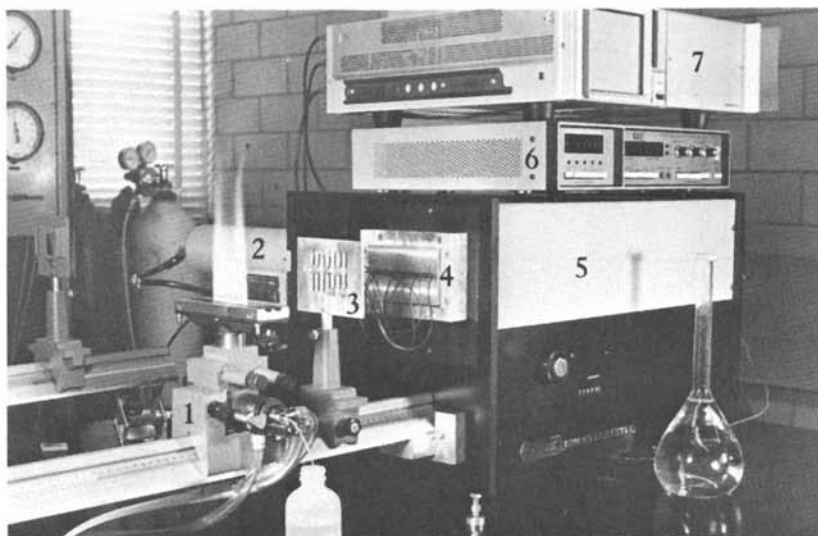
Figure 5. Fiber-optic vidicon spectrometer. (1) Nitrous oxide/acetylene flame; (2) SIT vidicon detector; (3) Fiber-optic input lenses; (4) Fiber-optic entrance slit system; (5) 0.5-m Czerny-Turner monochromator; (6) Optical multichannel analyzer; (7) Oscilloscope display.
